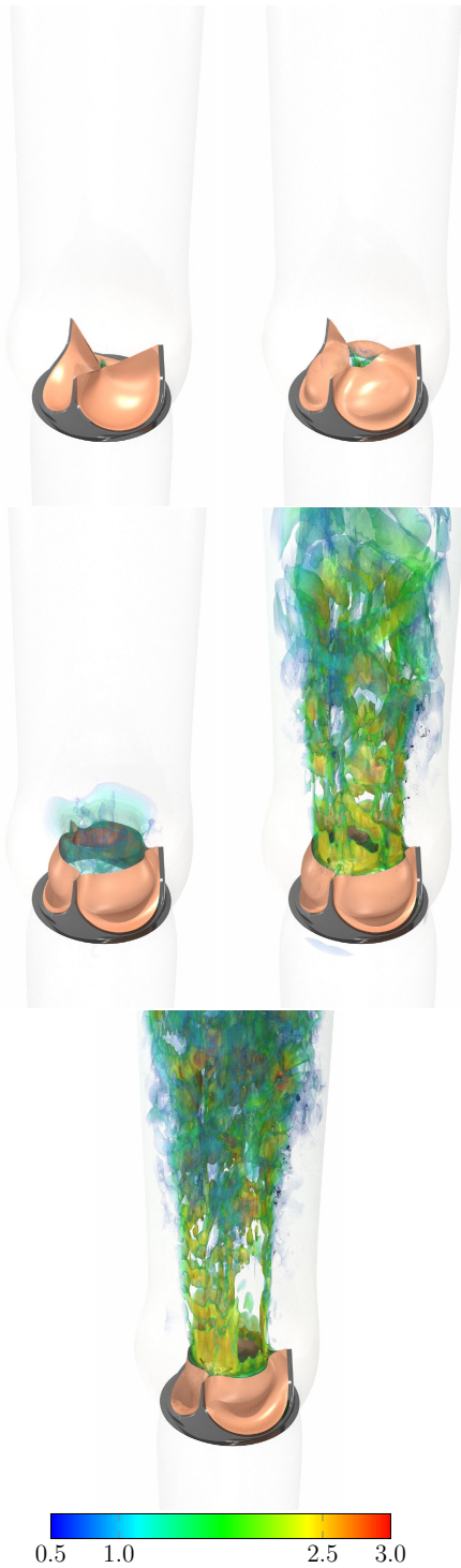
Fig. 12: Flow analysis of a BHV. Isosurfaces corresponding to a positive value of the second invariant of the velocity gradient tensor, colored by the velocity magnitude (m/s), at t = 1.035, 1.135, 1.175, 1.355, 1.445 s.
