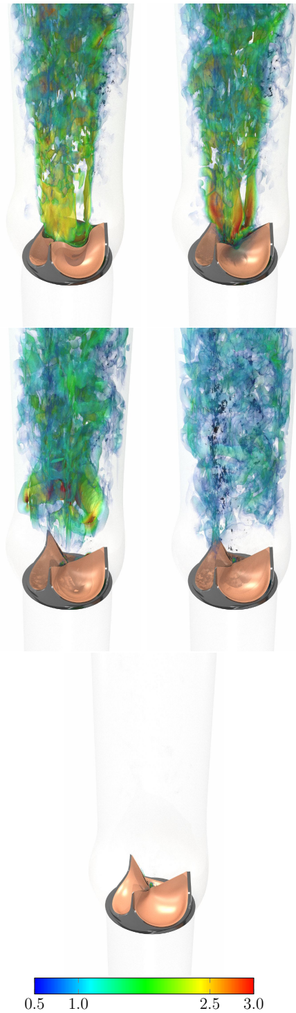
Fig. 13: Flow analysis of a BHV. Isosurfaces corresponding to a positive value of the second invariant of the velocity gradient tensor, colored by the velocity magnitude (m/s), at t = 1.450, 1.455, 1.465, 1.495, 1.645 s.
