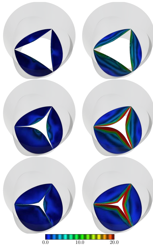
Fig. 15: Aortic-valve flow analysis. Asymmetric leaflet motion. Magnitude of the WSS (Pa). Upper surface ( left ) and lower surface ( right ). The frames are for t = 0.804 , 0.984 , and 1.028 s.
