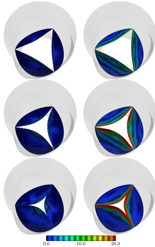
Fig. 11: Aortic-valve flow analysis. Symmetric leaflet motion. Magnitude of the WSS (Pa). Upper surface ( left ) and lower surface ( right ). The frames are for t = 0.804, 0.984, and 1.028 s.
