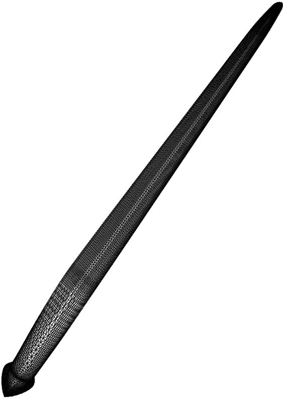
**Fig. 7** Rotor surface mesh.
