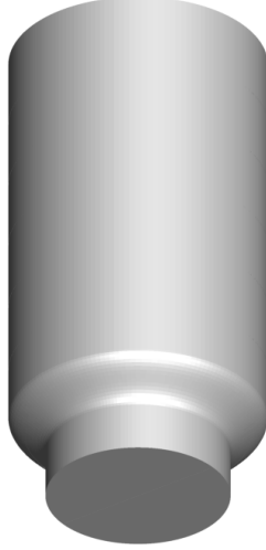
Figure 33: The shape of the fluid subproblem domain, \Omega_1 , defined by applying the transformation (239)–(241) to a trivariate B-spline parameter space.
