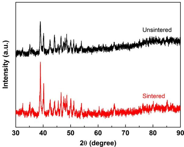
**Fig. 4** XRD spectrum for an un-sintered mixture sample of CNTs (0.5 wt.%) and chromium carbide powders (*upper*), and for a laser-sintered composite sample (*lower*)
