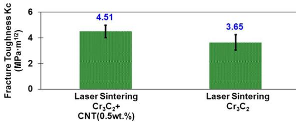
**Fig. 6** Vickers indentation fracture toughness of (1) composites produced by laser sintering of chromium carbide powders+CNTs (0.5 wt.%), and (2) material produced by laser sintering of chromium carbide powders without CNTs
