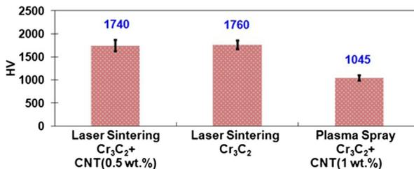
**Fig. 5** (1) Hardness of composites produced by laser sintering of chromium carbide powders+CNTs (0.5 wt.%), (2) hardness of material produced by laser sintering of chromium carbide powders without CNTs, and (3) hardness of composites produced by plasma spraying of chromium carbide powders+CNTs (1 wt.%) taken from [4]
