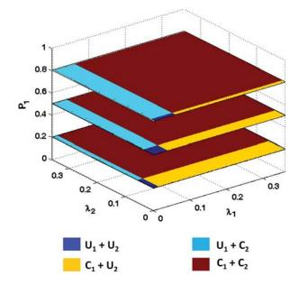
Fig. 7. Network phase diagram with two packet types. The transmission probability of packet type *i* is denoted as  $P_i$  under the constraint  $P_1 + P_2 = 1$ . The arrival rate for packets of type *i* is denoted at  $\lambda_i$ .
