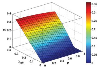
Fig. 5. Average (over time) packet drop rate (D) as a function of packet arrival rate  $(\lambda_{eff})$  and transmission probability (P).
