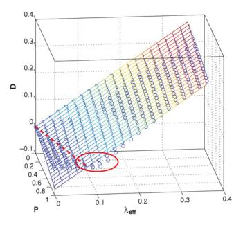
Fig. 8. Approximation of average (over time) packet drop rate (D) as a function of packet arrival rate  $(\lambda_{eff})$  and transmission probability (P) in square-grid networks. (Note: The region for D < 0 is inaccessible because the packet drop rate is nonnegative.)
