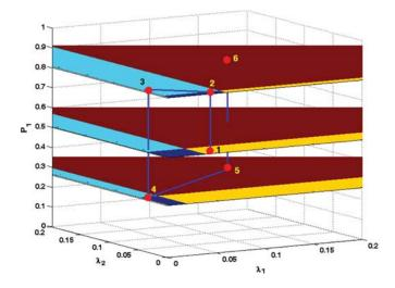
Fig. 9. System trajectory in the phase diagram for the representative experimentation. The transmission probability of packet type i is denoted as  $P_i$  under the constraint  $P_1 + P_2 = 1$ . The arrival rate for packets of type i is denoted at  $\lambda_i$ .
