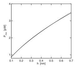
FIG. 1. The variation in the maximum power dissipated  $P_{\text{max}}$  with the thickness of the capillary layer h. The solid line is the exact result. The dashed line is a curve fit given by  $P_{\text{max}} \approx 4.5 h^{0.71}$ .
