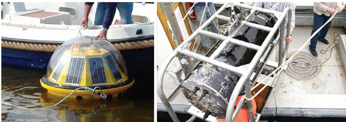
**Figure 4.** The left photo depicts a CytoSense benchtop scanning flow cytometer which is transformed into a CytoBuoy for moored operation. The right photo shows researchers lowering the FlowCytobot onto the WHOI research vessel *Mytilus* for deployment at the Martha's Vineyard Coastal Observatory (Photo courtesy Tom Kleindinst).<sup>87,88</sup>
