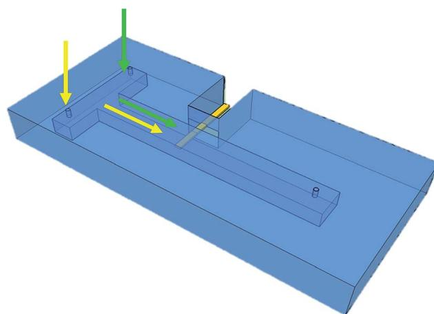
Fig. 1 (a) Schematic of assembled microfluidic mixing device (not to scale). Flow directions as shown. The actuator acts in a transverse direction to the fluid flow (in the z-direction as shown in this schematic).
