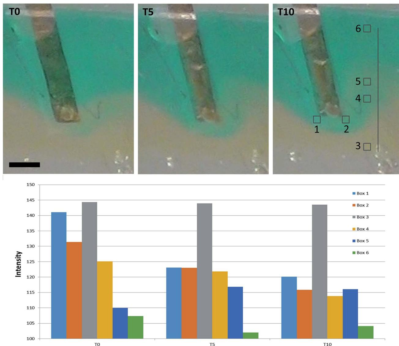
Fig. 3 Top right: Reference image at T10 of selected pixel regions used for analysis. Plot of mean intensity values generated from histograms of the labeled boxes 1–6 ( $10 \times 10$  pixel areas) shown in T10. Lower intensity values correspond to darker colors (green) in the images and higher intensity values correspond to brighter colors (yellow). Reference images for T0 and T5 are also shown; identical box scheme was used for analysis. Scale bar is 1 mm.
