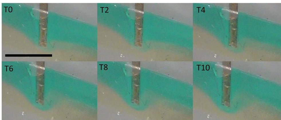
Fig. 2 Time lapse from T0 (where T0 represents time 0 s when the actuator was activated) to T10 of the channel area immediately surrounding the actuator. Flow direction is from left to right across the images. Scale bar is 5 mm.
