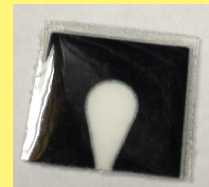
(Left) A completed microfluidic device with lamination. Blood enters via the open path on the bottom portion.
