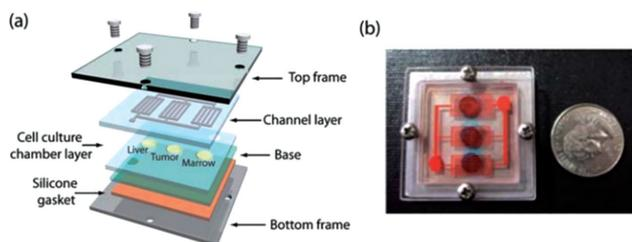
**Figure 12.** Layout of the device, showing A) the layer-by-layer design, and B) the image of the assembled device, with a quarter for scale. Reproduced with permission.<sup>[83]</sup> Copyright 2010, The Royal Society of Chemistry.
