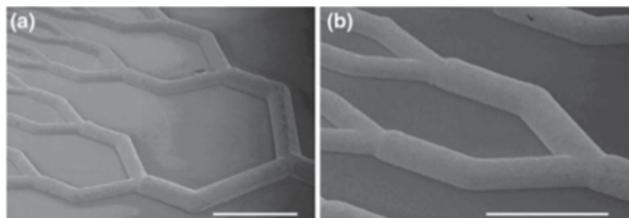
**Figure 9.** Image of the device. A network of bifurcating channels, each level containing a diameter smaller than the last, is shown. The scale bar is displayed at A) 1 mm and B) 500  $\mu\text{m}$ . Reproduced with permission.<sup>[65]</sup> Copyright 2009, Springer.
