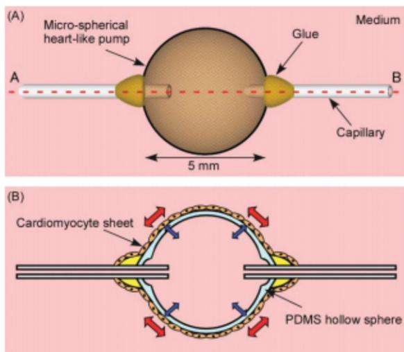
**Figure 8.** Diagram of the micro spherical heart pump, shown in A) a full view, displaying the components of the device and medium brought in through port A and expelled through port B. Additionally, B) a cross-sectional view is shown. The layer containing the rat cardiomyocytes can be seen, with red arrows shown to display their contracting nature on top of the PDMS sphere. Reproduced with permission.<sup>[60]</sup> Copyright 2007, The Royal Society of Chemistry.
